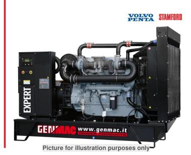
G450VO **Overall performance** PRP Continuous power kVA 450 PRP Continuous power kW 360 LTP Stand-by power kVA 500 LTP stand-by power kW 400 0.8 Power factor cos fiq Voltage VAC 400/230 Frequency Hz 50 Ampere PRP/LTP 650 / 723 Speed RPM 1500
